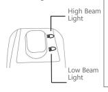
Remarks: To signal overtaking, the rider may press and hold the Pass button to enable the High Beam Light and Low Beam Light Interchange Mode. Release the Pass button to return to the Low Beam Light.
